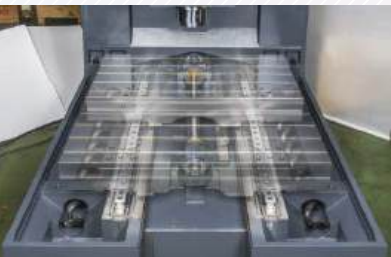
// Work Table is Full-travel Supported by The Base
